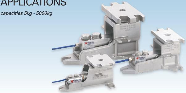
The LeverMount® is a unique, well-established load cell weighing assembly that makes installation much simpler, safer and more cost-effective than traditional assemblies. Its innovative design allows for fast load cell installation without any jacking tools or dummy (false) load cells – even with a loaded tank/hopper. It is available in 3 sizes, with reference to the load cell capacity: LeverMount® Lite (5-200kg), LeverMount® 300-2500kg and LeverMount® 3000-5000kg.
