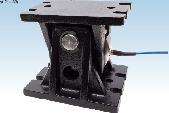
The T95 weighing assembly comprises a stainless steel high accuracy load cell, complete with a tough mounting accessory in painted alloy steel (optionally stainless steel up to 10t). Although the assembly is used in compression, the cell is mounted in a unique pendulum configuration and loaded in tension. This ensures that the load vector is always maintained through the central axis of the load cell, even when the assembly is subjected to considerable movement or misalignment.
