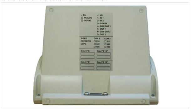
Figure 8.1 - Outputs identification label on base of terminal (citi0410.jpg)
